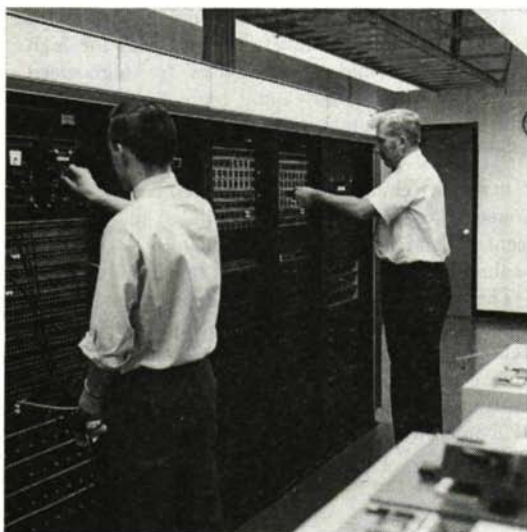
Master control board of the computer-controlled transmission system at CNT's Data Central, Toronto, the present major function of which is the handling of airline and railway reservations. The network is also used by the Meteorological Branch of the Department of Transport to transmit weather maps across the country for instant weather information.
